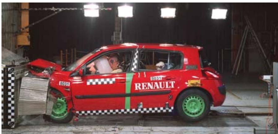
TrackImage calculates the dynamic parameters of the test: positions, speeds, accelerations, distances, angles, etc
